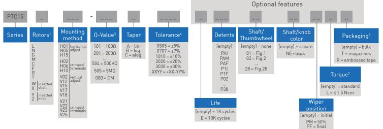
1. Rotors: "Z" adjustment only available on "H"-mounting versions. Color for "T" rotor is Orange.
