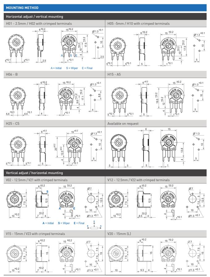
15-mm carbon / cermet through-hole potentiometer
